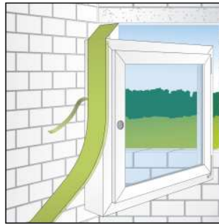
Fig. 1 Remove protective paper liner & locate tape to edge of frame with self-adhesive
