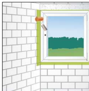
Fig. 3 Consolidate bond by rolling
