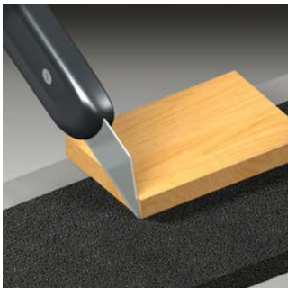
Figure 3: To accommodate setting blocks, notch out tape
