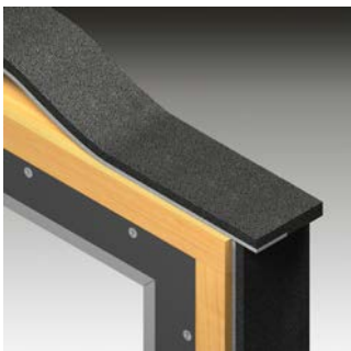
Figure 5: Apply the tape to the head and two sides of the window
