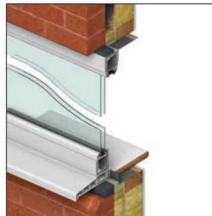
Fig 1 Location of TP450 Compriband Timber Max at initial installation
