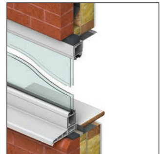
Fig 2 Expansion and compression of TP450 Compriband Timber Max after frame movement
