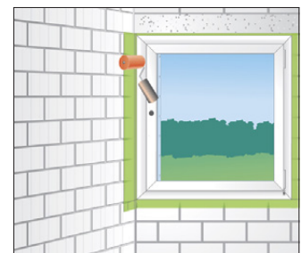
Fig 4 Consolidate the butyl bond using a roller
