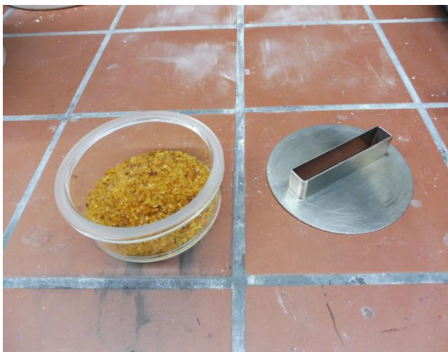
Figure 1: testing cup with Silicagel sorbent (left) and test template (right)
