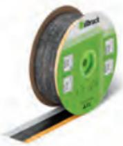
ME500 is a tearproof non-woven fleece fabric with a polyethylene copolymer film, including an integrated movement pleat for variable joint sizes and absorption of movement, and acrylic and butyl self adhesive strips for quick and easy installation.
