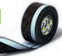
A variant of ME500, ME508 offers similar performance but with a fully faced acrylic adhesive layer, and no movement pleat. This provides excellent adhesion to most common building materials and ensures the membrane is bonded across the full width making it ideal if wet plaster is to be applied directly onto the membrane. Initial grab is sufficient to hold the membrane in place, but initial re-positioning is possible. The maximum bond strength is realised after around 24 to 48 hours.
