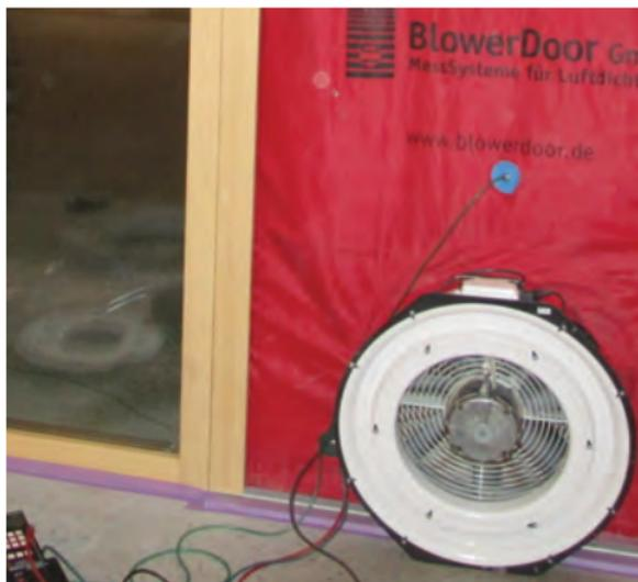
On-site air-leakage testing
