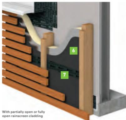
With partially open or fully open rainscreen cladding
