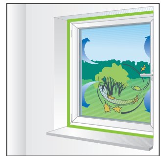
Fig 2 Seals against draughts
