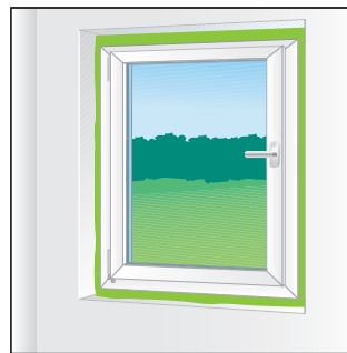
Fig 1 For the perimeter sealing of windows & doors
