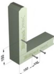
[Translate to Schweiz (Deutsch):] Centric screw spacing of 10 cm doubles the single screw load capacity.
