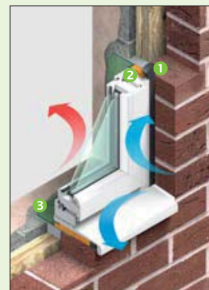
Traditional casement window detail with the i3 system
