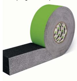
TP651 is an impregnated, pre-compressed multi-functional sealing tape. It is used for sealing the joints of windows and doors against driving rain and provides airtightness. It also offers thermal insulating properties within the perimeter gap between window and reveal and maintains the energy rating of the window/door.
