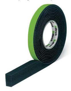
TP610 Duo is an impregnated foam tape which can be used for weather tight sealing of perimeter joints around windows and doors. In order to provide thermal insulation within the perimeter joint and maintain the energy rating of the window, it is recommended to also use FM330 Pro Foam Air Seal.
